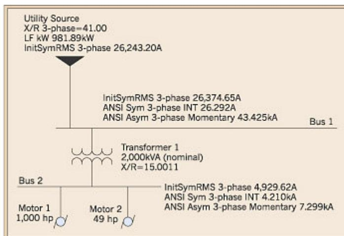
This over-simplified one-line diagram of a power distribution system included values necessary for working through the two methods of short-circuit calculation referred to in the text.
