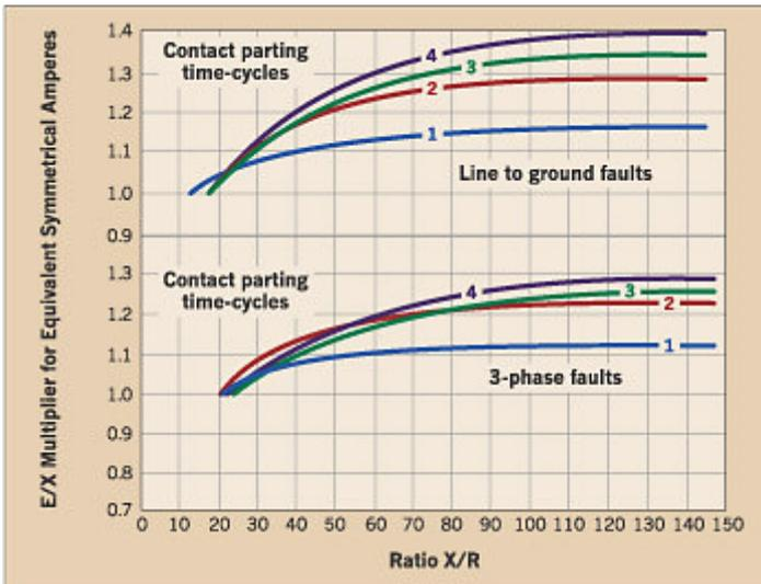
Multipliers necessary for one short-circuit calculation method are shown in ANSI C37.010-1999.
