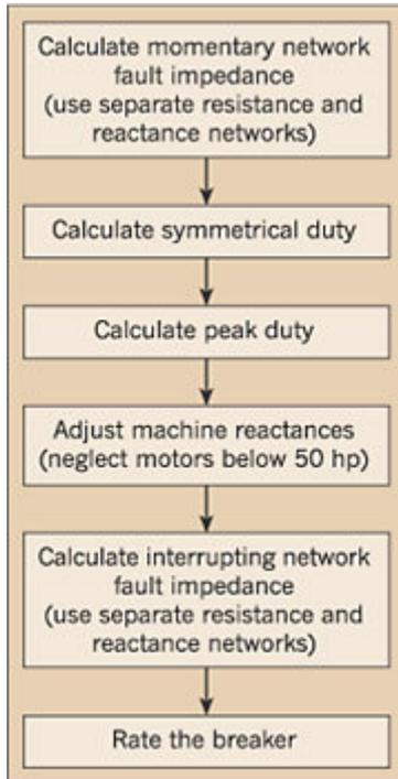
The ANSI/IEEE short-circuit calculation method follows a step-by-step process.
